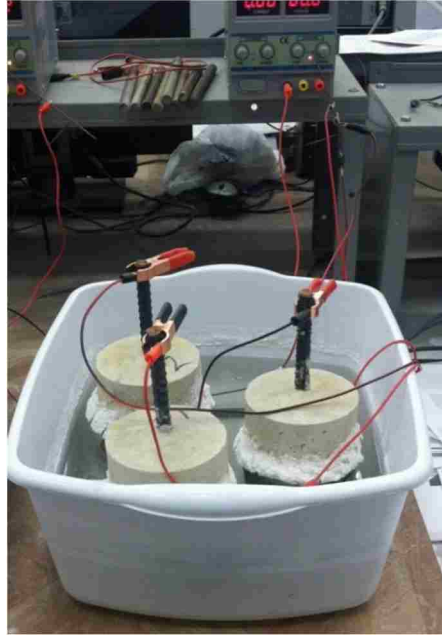
Figure 3.23 Corrosion test setup
