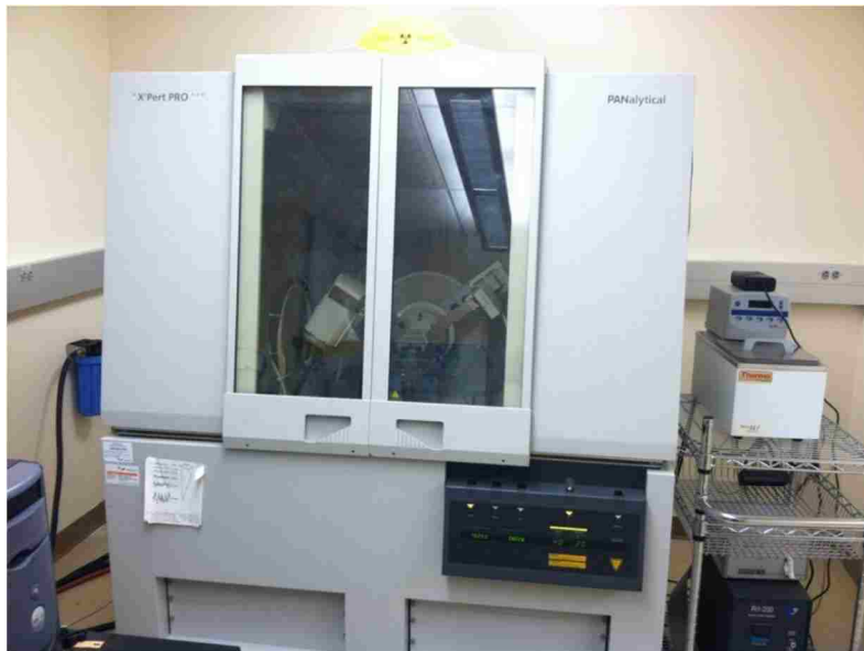
Figure 3.14 PANalytical X-ray diffractometer
