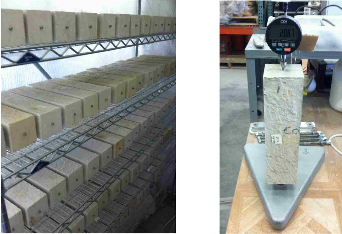
Figure 3.22 Shrinkage samples and dial gauge
