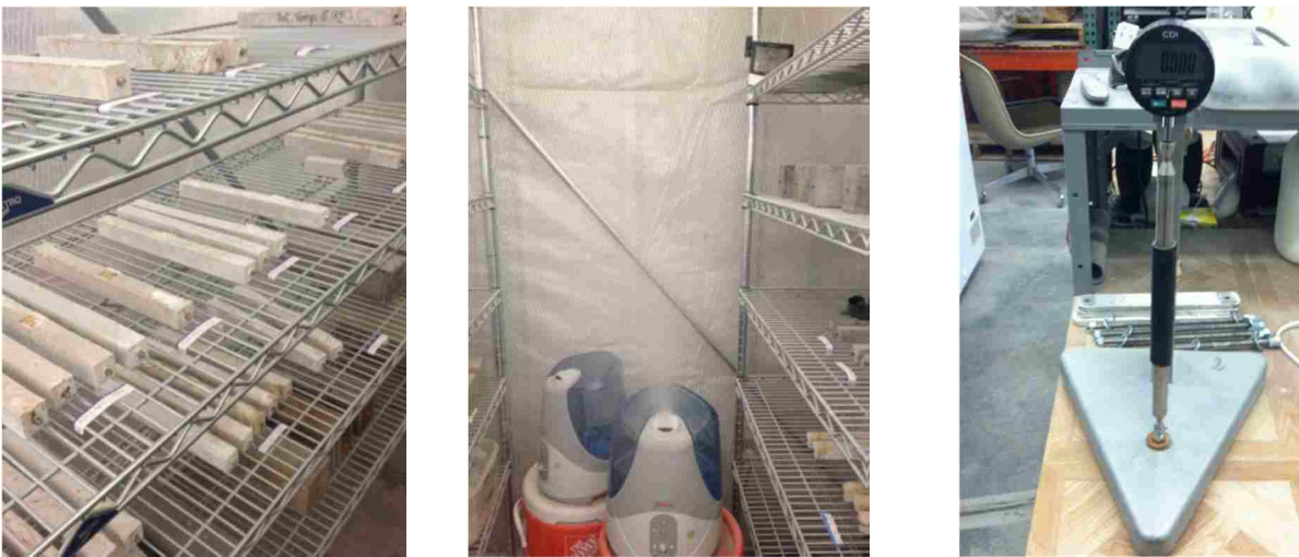
Figure 3.11 Humidity chamber (shrinkage room), drying shrinkage samples and dial gauge
