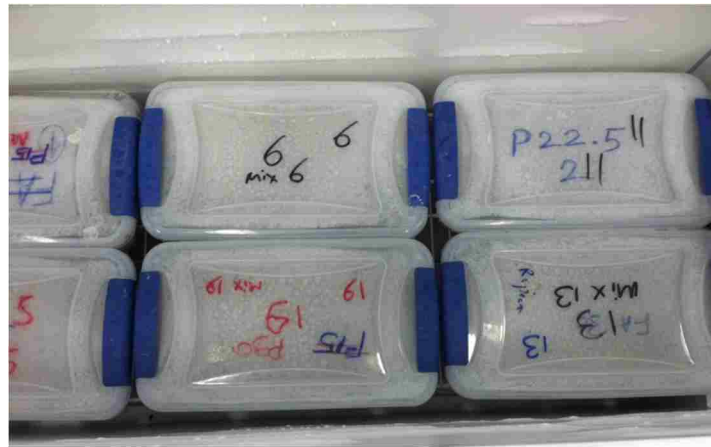
Figure 3.25 Freezer and samples in freezing and thawing cycle
