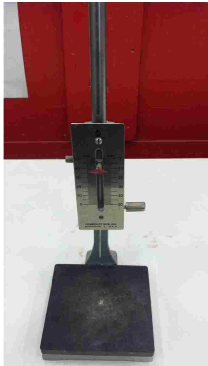
Figure 3.8 Setting time test device
