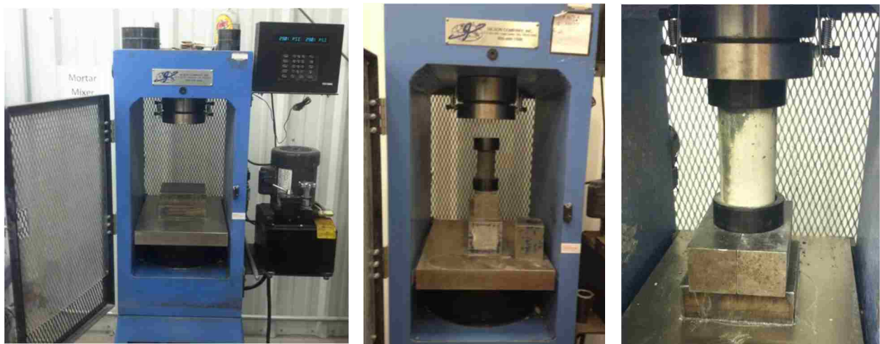
Figure 3.10 Compressive strength test setup
