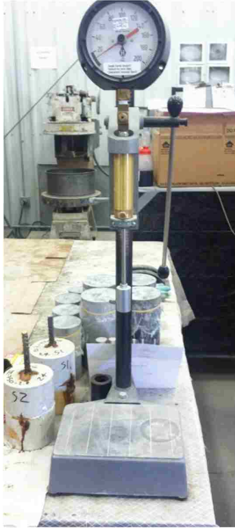
Figure 3.19 Setting time test device for concrete
